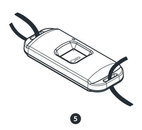
Use zip ties to attach the range extender in the desired location.
