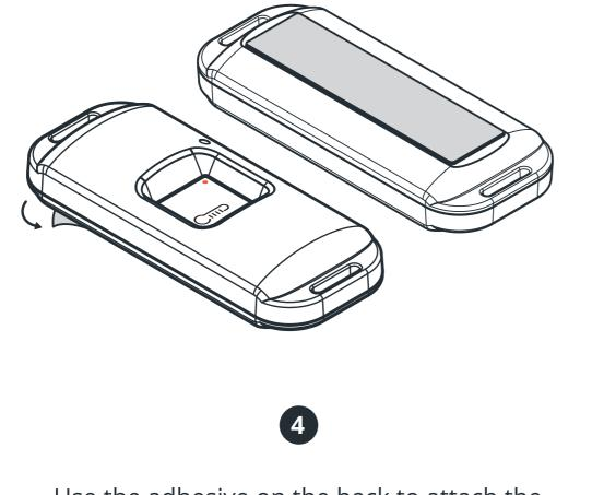
Use the adhesive on the back to attach the range extender in the desired location.
