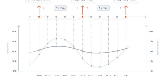
Events for a sensor configured to 3 minute measurement interval and 15 minute heartbeat.
